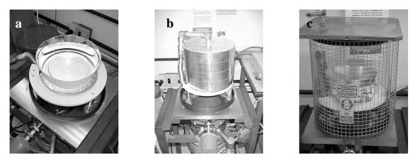
Figure 6 – a) Triple stage PCR mounting; b)  $LN_2$  shroud and vacuum system; c) Experimental mounting inside the bell jar.
